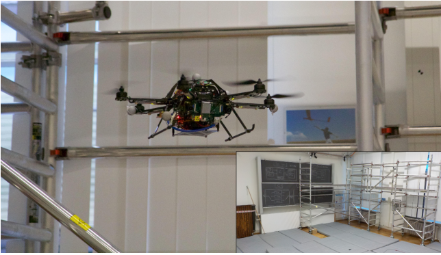
Fig. 7: The AscTec Firefly hexacopter MAV is depicted, together with the scaffold structure used for the exploration experiment.
