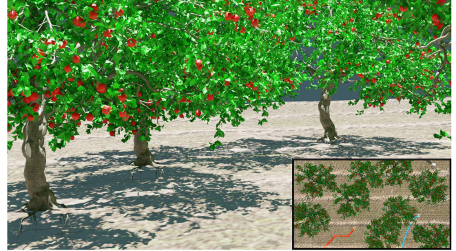
Fig. 1. View of one of two drones exploring a synthetic forest with geometrically realistic tree models. The inset depicts the top view of the scene of the experiment and parts of the robots' trajectories. The proposed system guides the safe and successful exploration of the digital model of the forest by the two UAVs. The planner is able to avoid collisions between the UAVs and the scene while clearing frontiers on the go by balancing cautious and aggressive navigation in a bid to maximize the efficiency of the exploration. Coordination is achieved in a decentralized fashion, relying on direct peer-to-peer communication.
