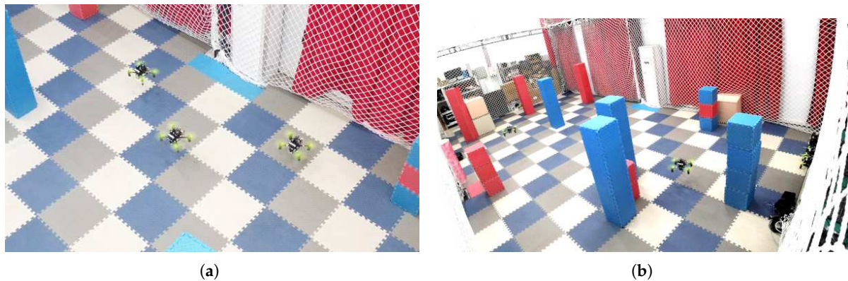
Figure 8. The practical experiments. (a) shows the initial status of three UAVs; they are placed on the same side of a room. (b) shows three UAVs are performing exploration in one trial; a 10 \times 8 \times 3 \text{ m}^3 virtual boundary is set to bound the exploring space.
