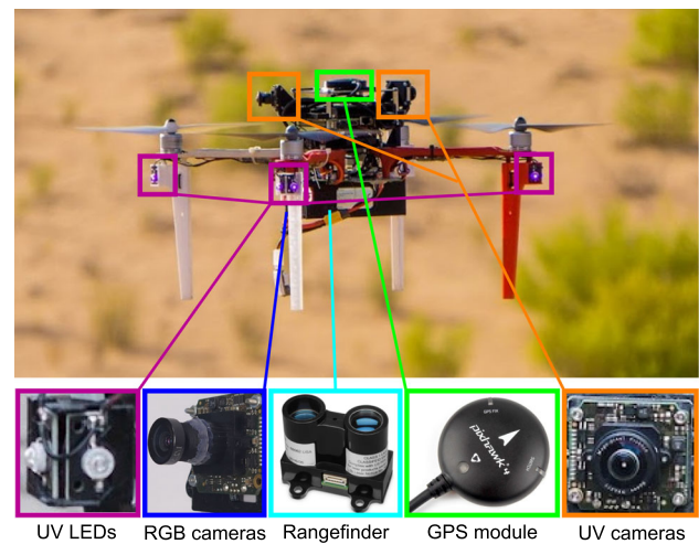
Fig. 5 Sensory equipment of the aerial vehicles used for experimental verification
